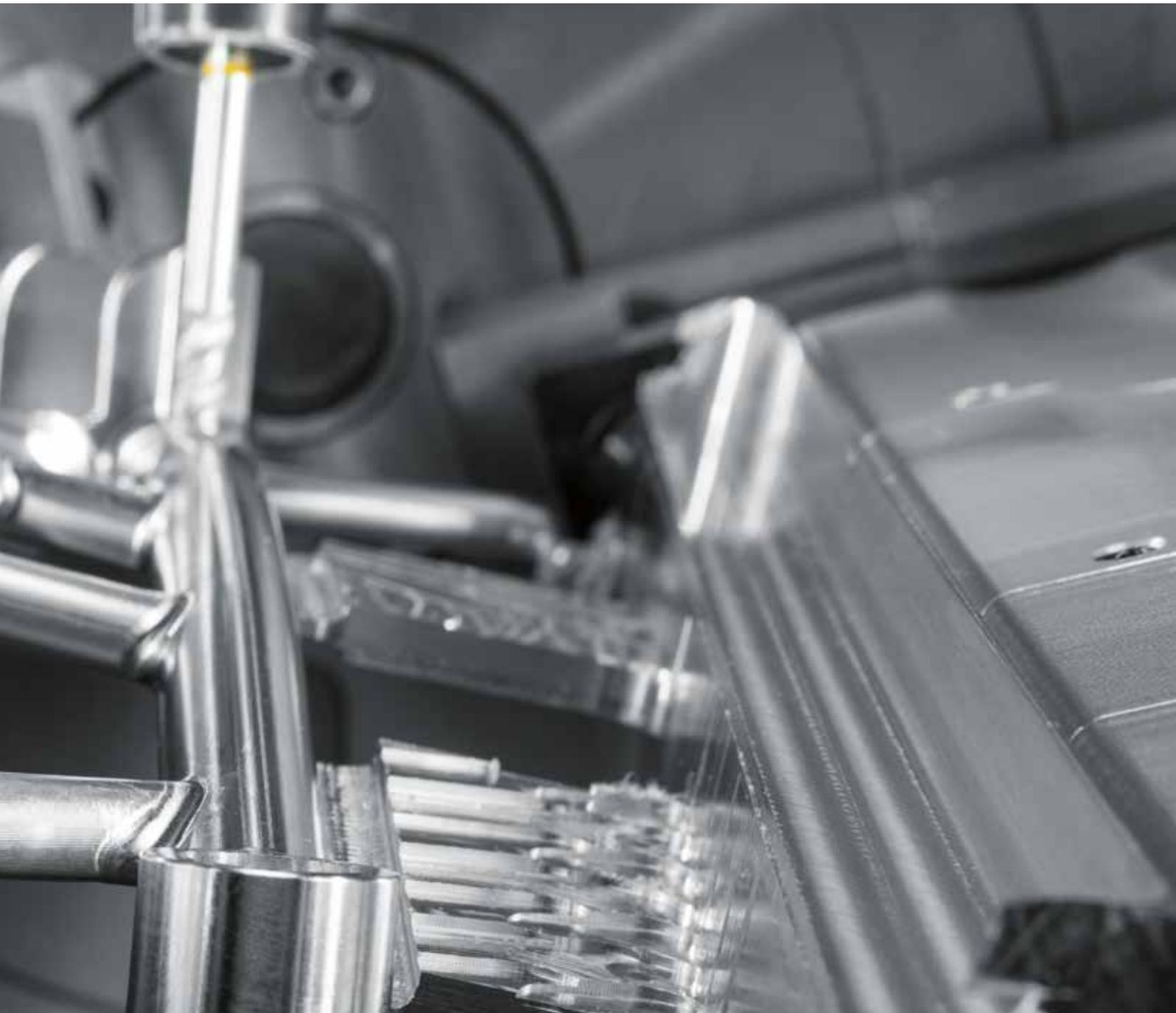
Automotive engineering. Frame section of an aluminum footrest support for a motorcycle. Complex 5-axis full-machining milling process – for extreme demands in racing.
