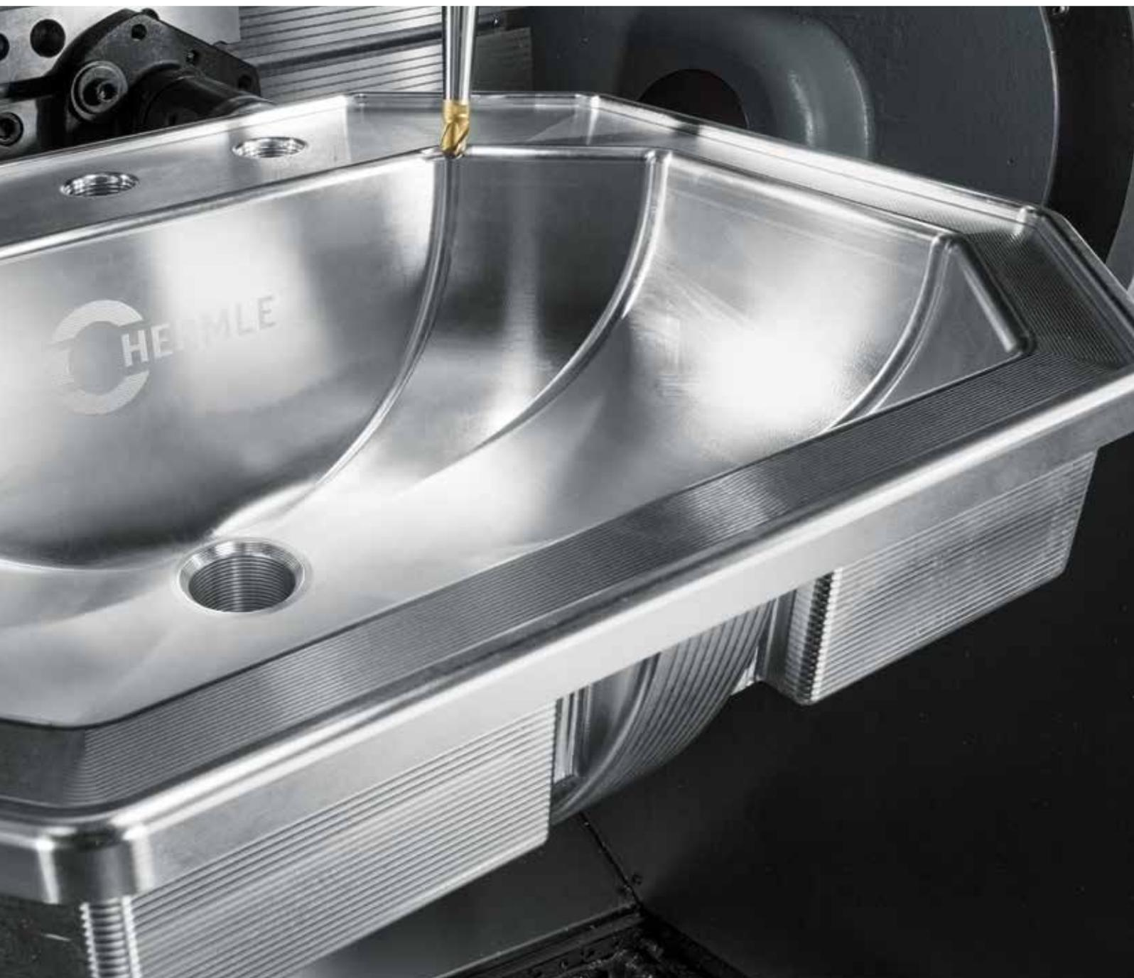
Model making. A hand washbasin for prototyping in aluminum.
