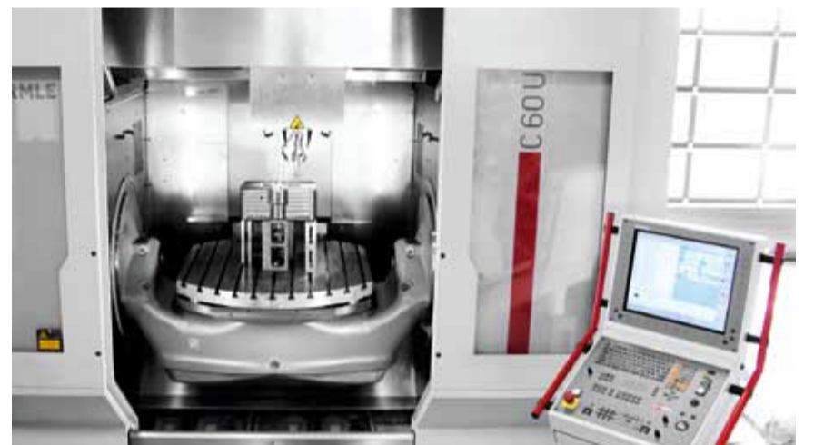
Overall view of a 5-axis high-performance CNC C 60 U machining center from Hermle with a working area of 1200 x 1300 x 900 mm (X, Y, Z), a tool magazine with 70 compartments and a Heidenhain iTNC 530 control.
