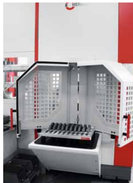
The RS2 setup station equipped for parallel pallet loading and unloading at primary machining times. MAWAtec’s own pallets for multiple uptake of raw-sawn or lasered blanks.
