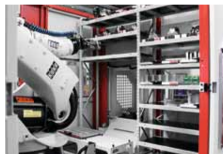
RS2 robot system with some of the heavy load racks for taking on pallets at varying heights; below left: the rear opening of the setup station.
