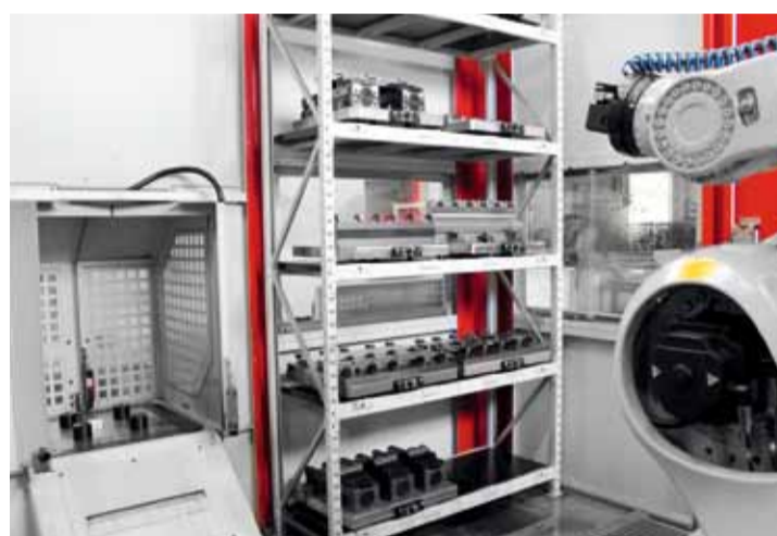
A flexible manufacturing system as an integrated unit with a C 40 (already active, on right) and an RS2 workpiece magazine and handling system (left); ready-prepared for the planned integration of a further C 40 U to be placed to the left of the RS2.
