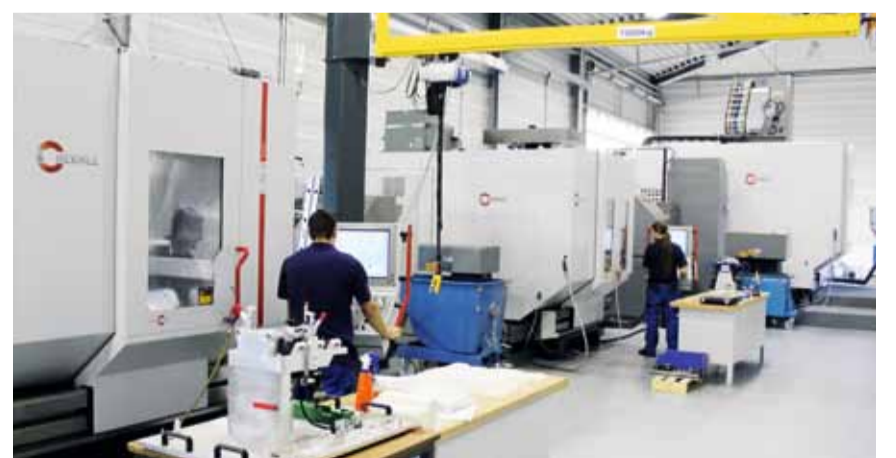
Deharde’s „Hermle Line“ with three of four Hermle machining centers – front C 22 U, center C 42 U, rear the C 60 U with the purpose-built „5-axis hall“.
