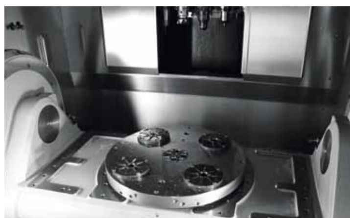
NC swiveling table with integrated 420 mm rotary table (allowing the Z-axis path to be retained) and added compact pallet receiver.
